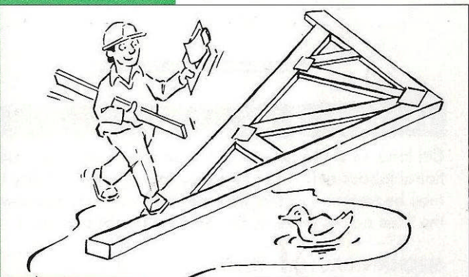
Bearers should be placed on a level, hard and dry surface. A waterproof covering must be used to protect components against rain and sun and allow good air circulation. In vertical storage, bearers must be high enough to keep rafter overhangs clear of the ground. In horizontal storage bearers must be arranged at close centres to give level support.
